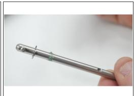
Apply grease around the shaft as shown in the photo.
