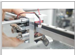
Affix the Back Plate to the X-Carriage using the four standoffs.
