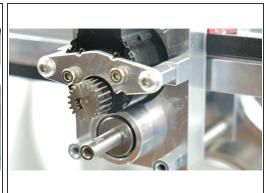
Slide the remaining bearing race onto the shaft.
