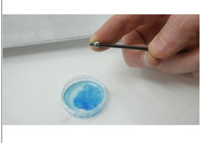
Apply Thread Lock to an M3 5mm Socket Cap Screw.
