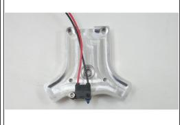
Attach the Endstop to the back of the Face Plate.
