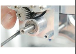
Slide the larger internal diameter bearing race onto the shaft with the groove facing outwards.
