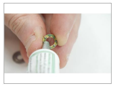
Flip the bearing pack and apply grease to the other side.
