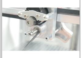
• Slide the MR1052ZZ bearing over the shaft and into the bearing pocket in the Back Plate.
