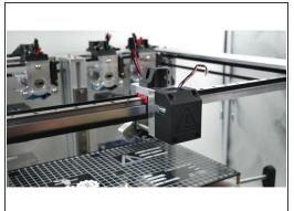
Attach the Printed X-Carriage Cable Bracket to the X-Carriage using two M3 8mm Socket Caps screws.
