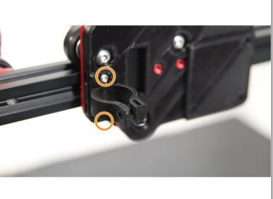
Both the Capacitive sensor and the BLtouch can be secured using 2 M3x5 screws (Same ones that were used to hold the hotend cover in place) against the two M3 square nuts inserted in the previous step
