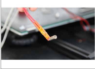
With a pair of side cutters or blade, cut the insulating tape around the heater cartridge and thermistor wires
