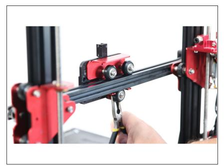
Once the carriage is back in place, use a pair of pliers to slowly turn the eccentric nut until there is no wobble left in the carriage
