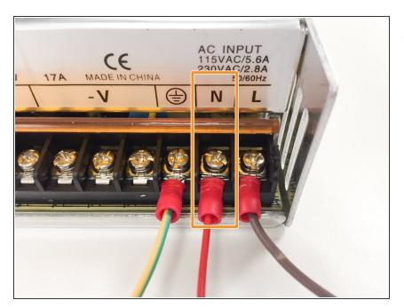
Connect the second red wire from the head bed into the neutral terminal of the power supply.
