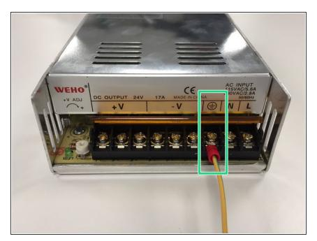
Connect the other end of the earth/ground wire to the power supply.
