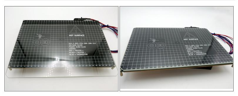
Place the Borosilicate glass on the Varipower bed.
