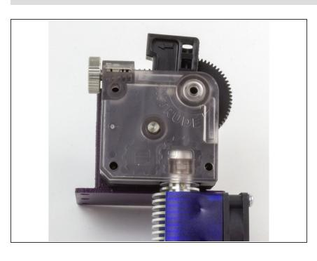
Press on the lid to your extruder. It should be flush with all the sides of the body.
