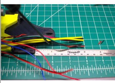
Trim wires 50-75mm longer than the top of the mount. This gives freedom to manage the wire connector for the TAZ 6.
