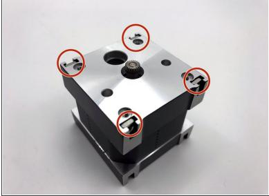
Place x4 M3 square nuts into the T slots on motor face.
