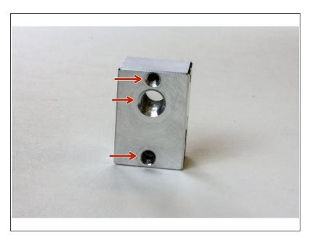
Triple check once again that you're about to screw your nozzle into the side of the heater block with three holes on it.
