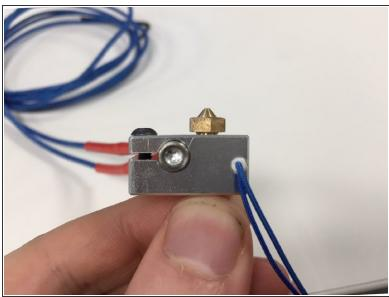
• Tighten the M3 x 10 socket dome screw (with the M3 washer on it) with 2 mm hey key until the clamp deforms slightly (as shown in the second picture).
