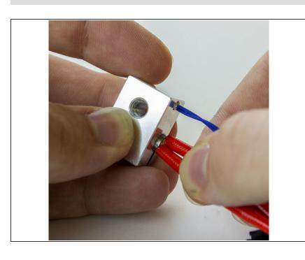
Before moving on, gently tug on your thermistor and heater cartridge wires. We don't want them slipping out during a print!
