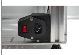
Secure the IEC with two M3 50mm Counter Sunk Screws.
