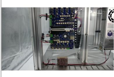
If you have opted to use the SSR use the two supplied Negative and Positive cables to connect between the Duet's Heated Bed screw terminals and the SSR's Input terminals.
