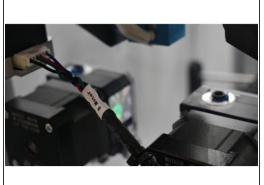
• Plug Motor B cable into the Left side Motor as looking from the back of the printer.
