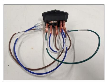
Connect the earth wire to the IEC housing as shown.
