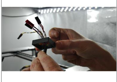
Remove the rectangle from the top of the tool and pass the T0 wires through it.
