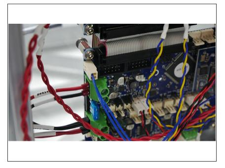
Plug the connector into the Bed Sensor Input on the Duet.
