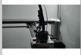
Secure the cables on the X-Carriage using Cable Ties.
