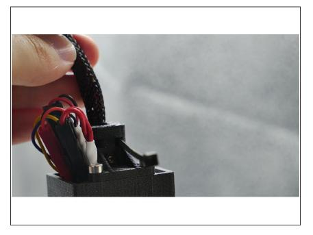
Secure the wires with a Cable Tie.
