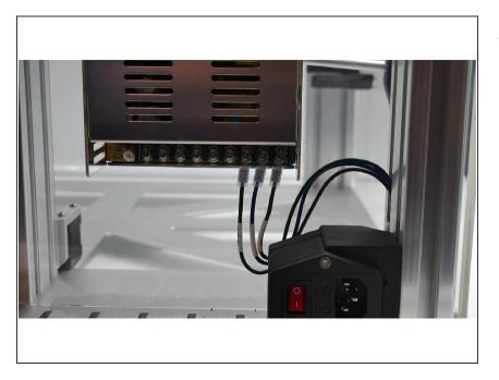
Correctly connected the PSU and IEC wiring should look like this.
