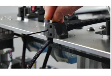
Insert a strip in the printed part and secure using the grub screw.
