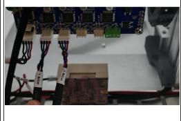
Plug in the motor cables.
