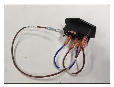
Connect the end of the brown wire to the switch as shown.
