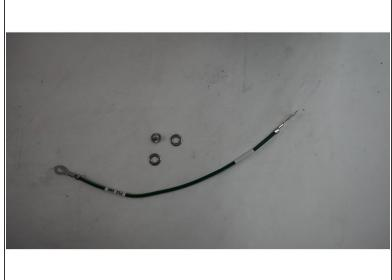
Find the short PSU to FRAME GND cable.
