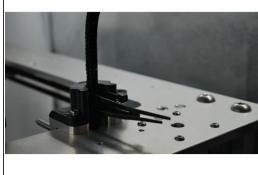
Pass two Cable Ties into the printed part for T0.
