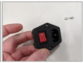
Insert the switch into the IEC Housing as shown.
