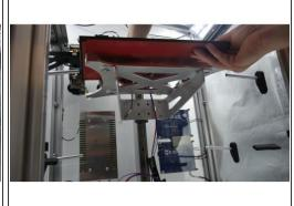
• Pass the Dragchain between the Bed Plate and Bed Bracket.
