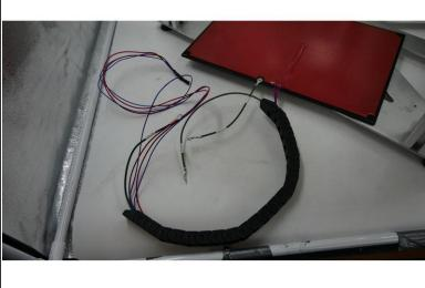
Feed the longer BED GND through the Dragchain.
