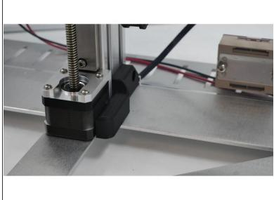
Affix the Printed Motor Cable Cover as shown.
