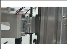
Reattach the Dragchain to the Bed assembly.
