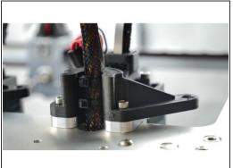
• When happy with the cable legnth use the two cable ties to secure the cable.
