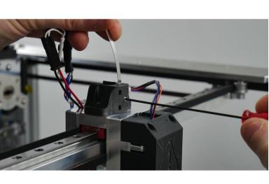
• Feed the strip through the braided sleeving and secure in the X-Carriage printed part using the grub screw.
