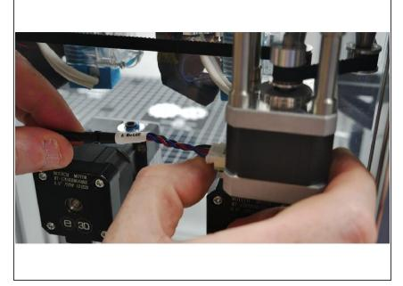
Plug the A Motor Cable into the right side motor.
